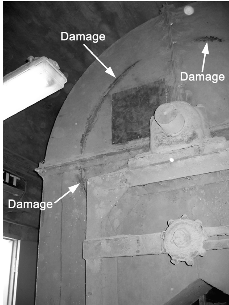
Figure 1 Examples of Damage to Bucket Elevator
