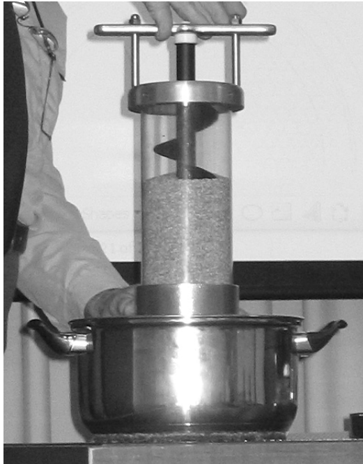
Figure 4 “Full-Bore” Flow of Material in an Olds Elevator Demonstration Unit
