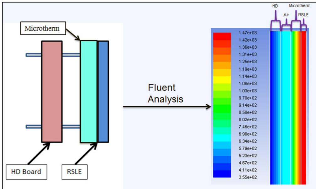
Fig 3. Cavity wall structure composition and thermal analysis (K)
