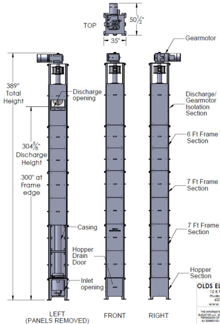
Fig 7. Design of the Olds particle elevator (dimension in inches)
