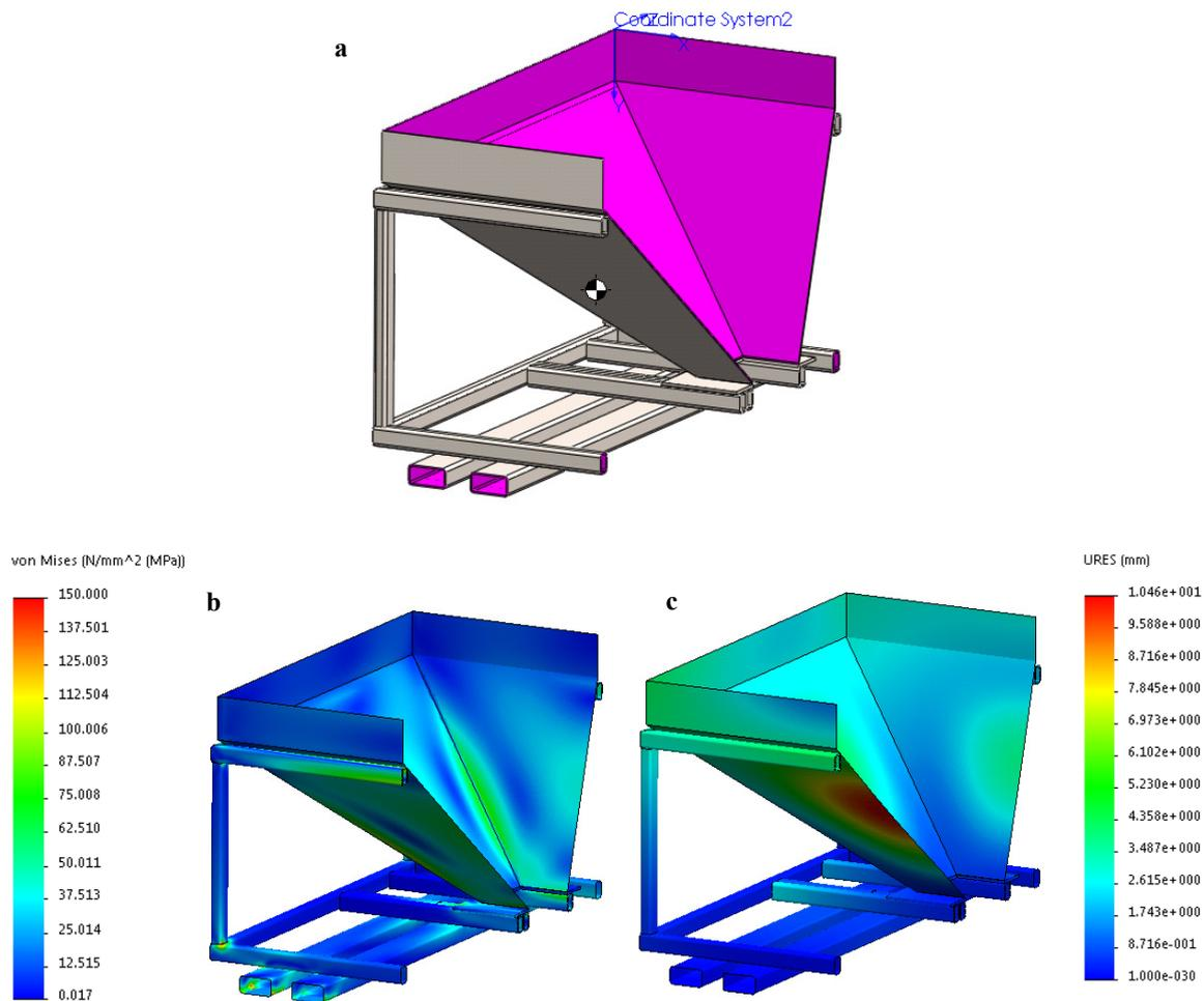
Fig 6. (a) Half-symmetric bottom hopper geometry, purple surfaces designating inside of hopper; (b) Stress (MPa) contours with thermal and dead loading; (c) Displacement (mm) contours with thermal and dead loading
