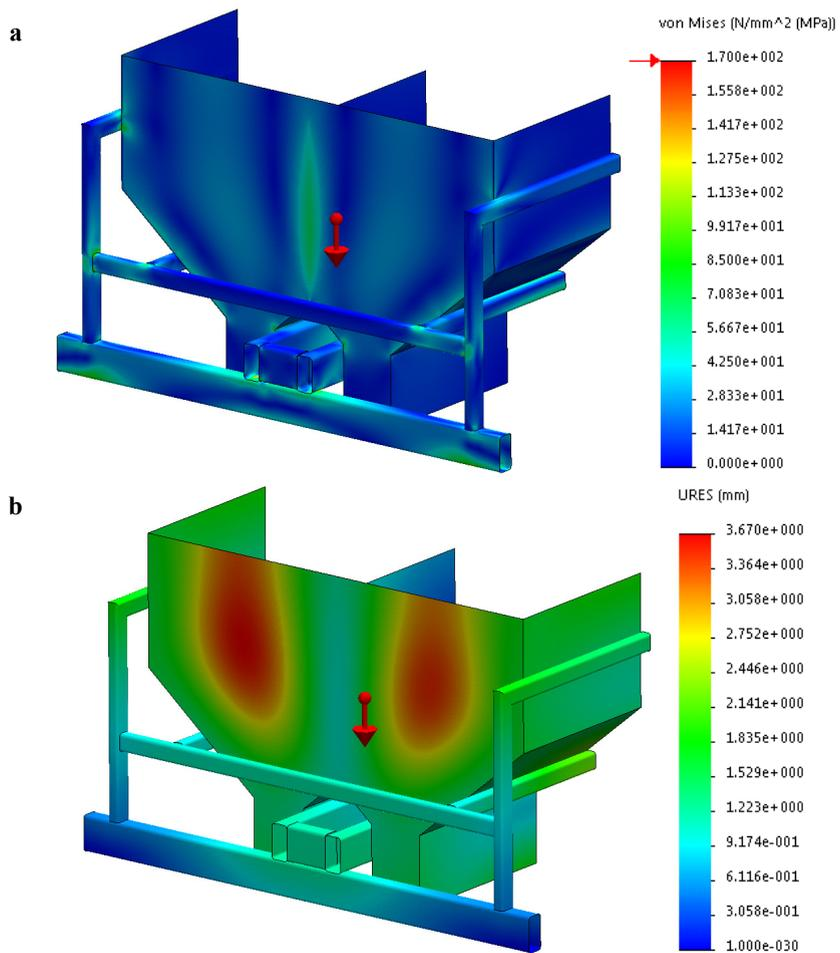
Fig 5. (a) Thermal and dead loading stresses (MPa) in top hopper; (b) Displacements (mm) in bottom hopper due to loading
