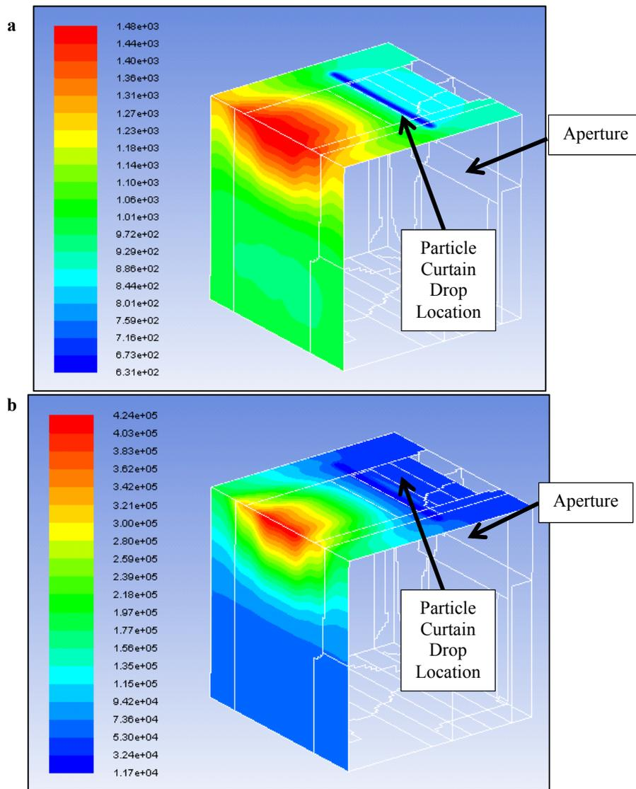
Fig 2. 2 m x 2 m x 2 m, 4 kg/s total particle mass flow rate, (a) Cavity wall temperatures (K) of top and back wall showing high temperature at the joint of the back and top walls; (b) Surface incident radiation (W/m<sup>2</sup>) on top and back wall showing the high flux concentration on the same joint with high temperatures
