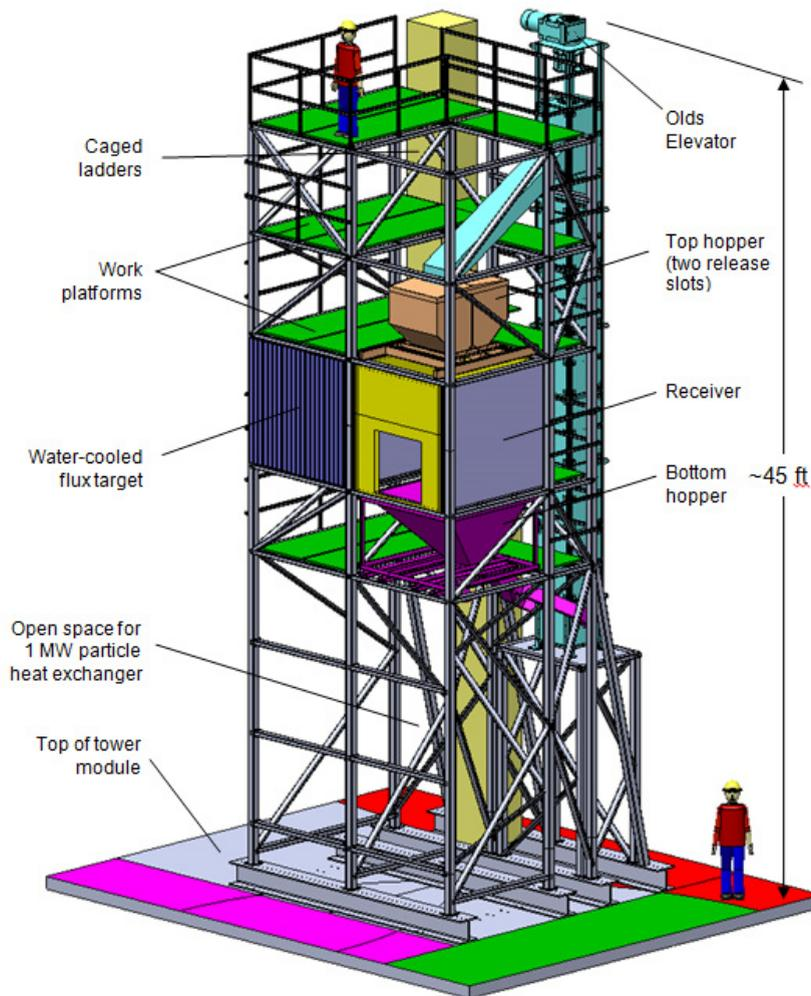
Fig 1. Prototype structure including work platforms and ladders (green and light yellow), bottom hopper (purple), top hopper (light brown), OLDS elevator (light blue), NSTTF module (multi-colored platform at the base; see Figure 1 for color codes). Heat shielding around the receiver and flux target is not shown. This system will be lifted on the module to the top of the 200 ft tower at Sandia's NSTTF.
