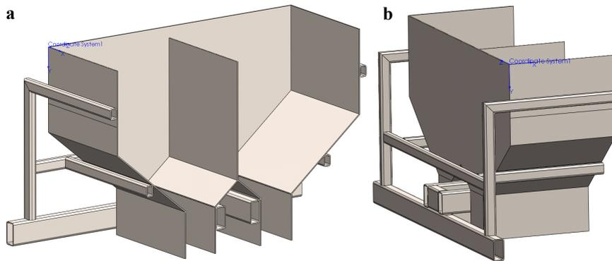
Fig 4. Top Hopper geometry, Isometric views showing inside (a) and outside (b) of symmetrical geometry
