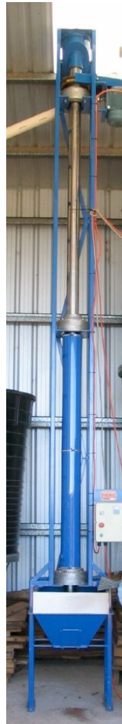
Figure 2 (left) – Macadamia nuts are gently elevated with this 100 mm (4") diameter Olds Elevator.
