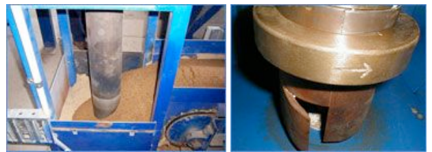
Figure 7 – The bulk material can be easily picked up near ground level (left), being fed by the two rotating in-feed pickup scoops at the base of the casing (right).
