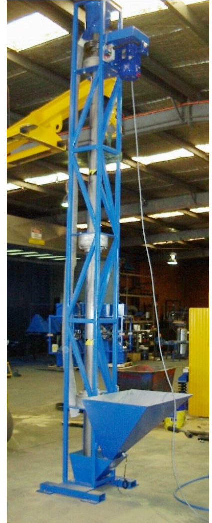
Figure 2 (left) – Macadamia nuts are gently elevated with this 100 mm (4") diameter Olds Elevator.
