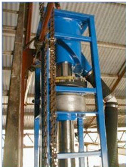
Figure 10 – Top of the 7.9m (26 foot) elevator being tested at Olds Engineering, showing discharge hopper, drive pulley, bearing, and Stainless steel 100mm (4") O.D. rotating tube.
