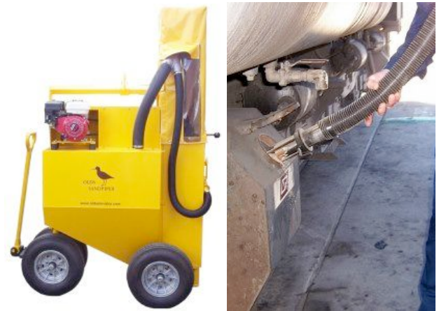
Figure 16 – The Sandpiper uses an Olds Elevator for refilling sand boxes in locomotives.
