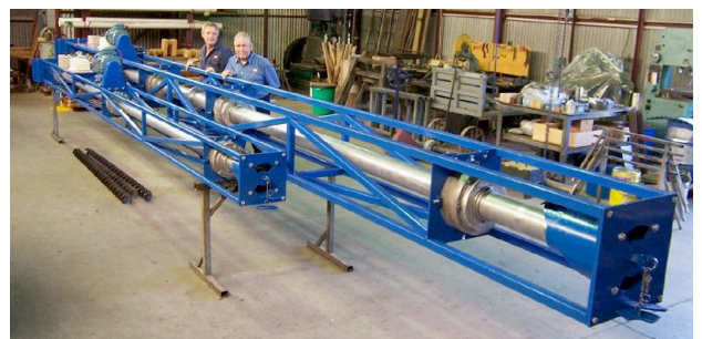
Figure 4 – Completed 100 mm (4") diameter and 152 mm (6") diameter by 10.7 metres lift Olds Elevators for Bean Growers Australia at Olds Engineering, Maryborough.
