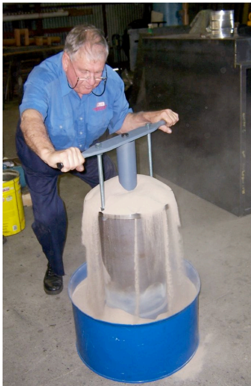
Figure 19 – 254 mm test Olds Elevator being rotated by hand delivers fine sand without any fall back through the 12.7 mm annular clearance gap.
